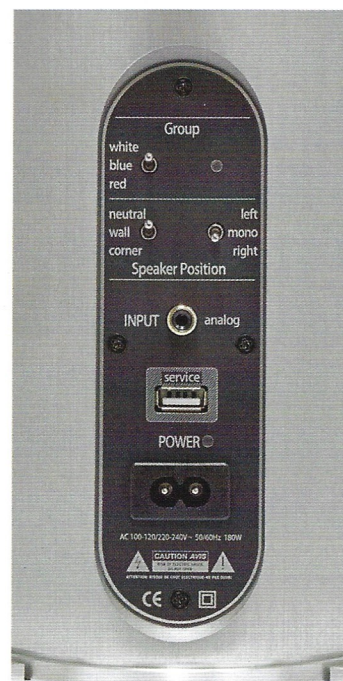
Toggle switches on the rear enable users to tailor the sound for the speaker position, or to be assigned to right or left channel, or mono mode. There is also an optional analogue input, via 3.5mm jack.
