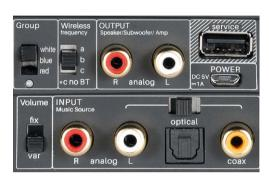
Using the "Hub", the Piega can be controlled either analog or digital via cable as well as "wirelessly". It can also be combined with a subwoofer.
