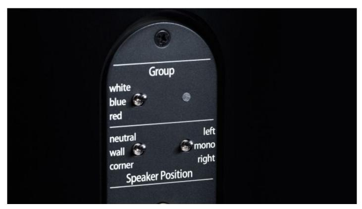
Switches on the back of the cabinet allow adjustment for speaker position and grouping them in a multiroom set-up (Image credit: Piega)
