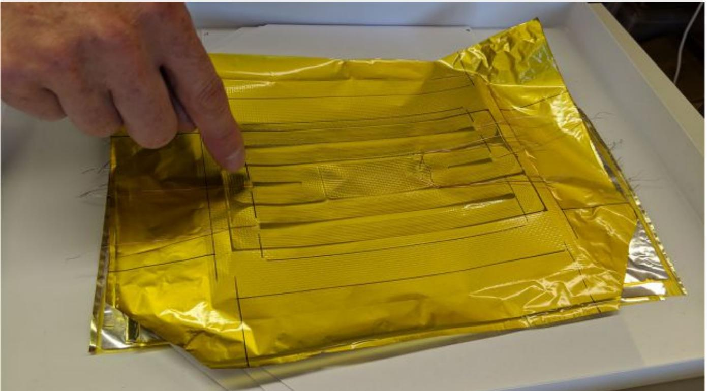
The corner room, where the ribbon tweeters are put together, is an oasis of relative calm. Life begins as a super-lightweight leaf of etched titanium voice coil. Replacing a dome tweeter on a conventional speaker is this 0.012g aluminium propathene sliver covered in a 0.007g foil supporting material.
