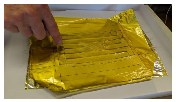
The corner room, where the ribbon tweeters are put together, is an oasis of relative calm. Life begins as a super-lightweight leaf of etched titanium voice coil. Replacing a dome tweeter on a conventional speaker is this 0.012g aluminium propathene sliver covered in a 0.007g foil supporting material.
