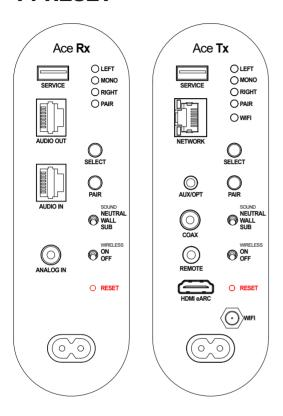
To perform a reset to factory default use a pointed object to push the «RESET» button on the rear panel of your speaker. The following settings will be deleted:
