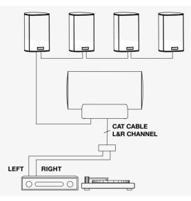
This expert setup reliably connects one or several speakers even via long signal lines. You will need the following devices:
