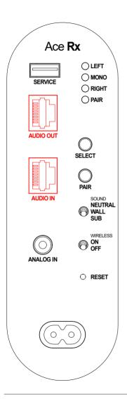
The Ace Rx speakers are equipped with a balanced analog input (stereo). The built-in RJ45 jacks allow for inexpensive and easy installation, and the signal can be routed via standard CAT network cables. It is imperative to use shielded cables and RJ45 plugs. The following graph provides an overview of the pin assignment of the RJ45 connector.
