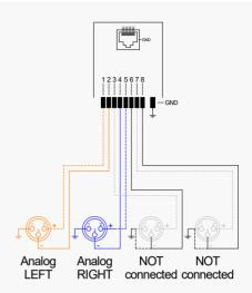
The signal is internally routed from RJ45 «AUDIO IN» to RJ45 «AUDIO OUT».
